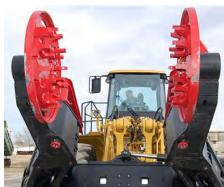
WBM Tire Handlers are designed to safely and efficiently handle OTR tires and rim assemblies on large mobile equipment.
